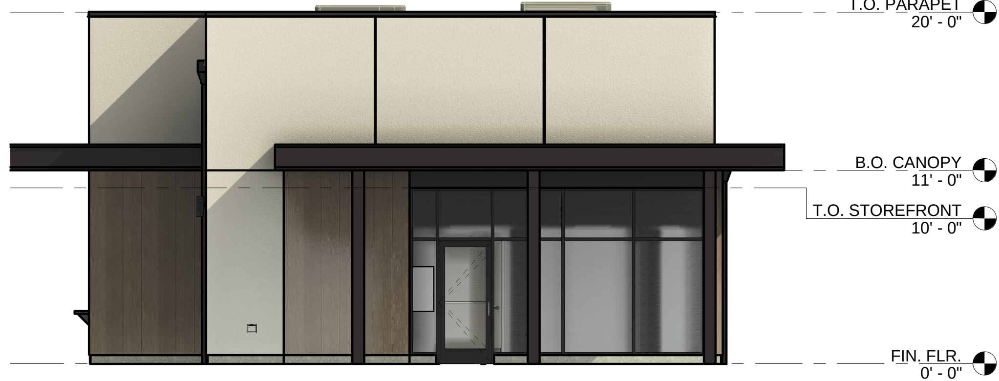
4 SOUTH ELEVATION PRELIM Scale 3/16" = 1'-0"
