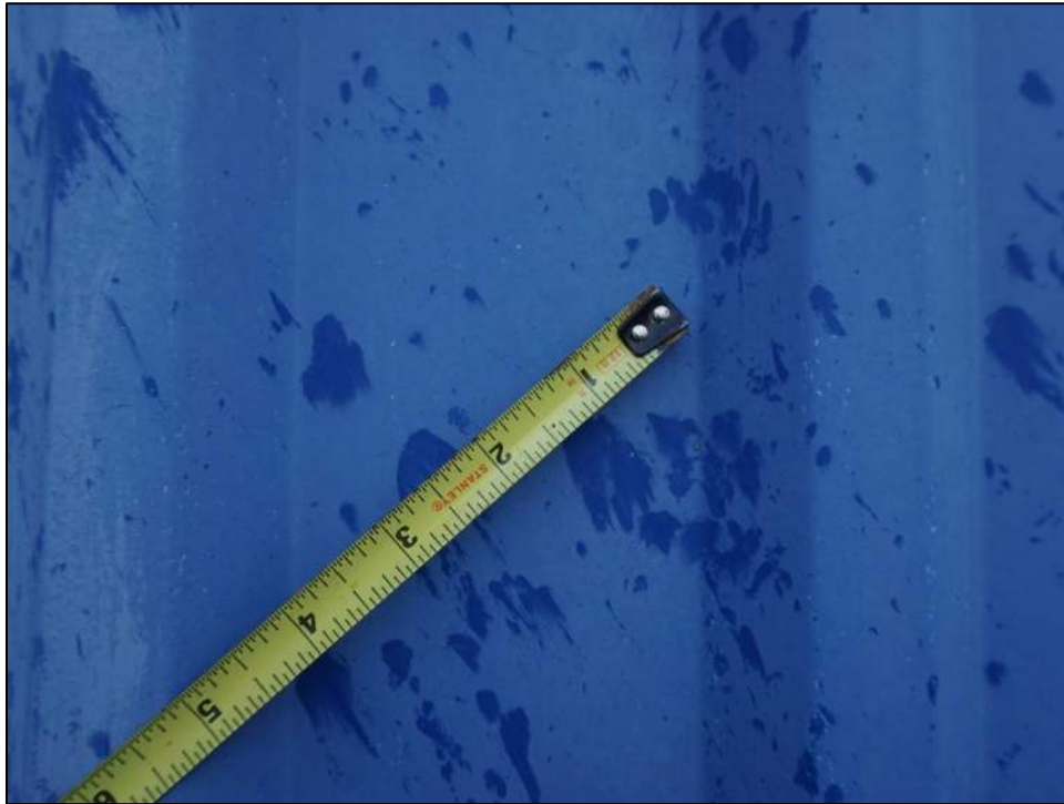
Photo 33: Largest hail spatter reflect hail of 1.5-inch hail.
