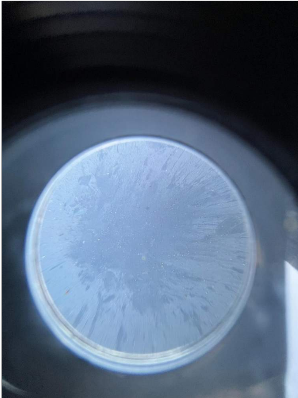
Photo 18: Microscope inspection indicated no coating disruption at hail dents or spatters.
