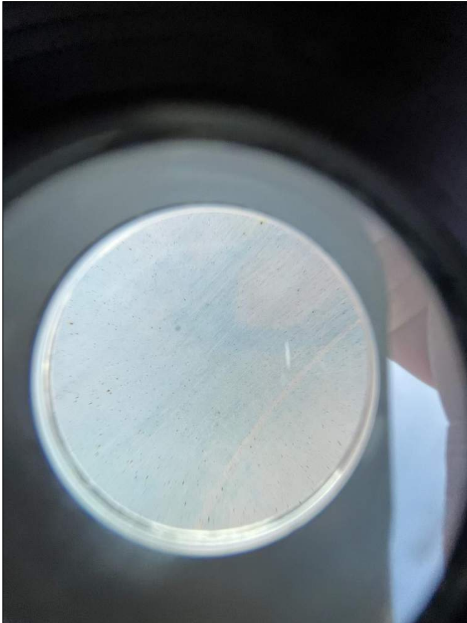
Photo 22: No coating disruptions were observed at the hail dents.
