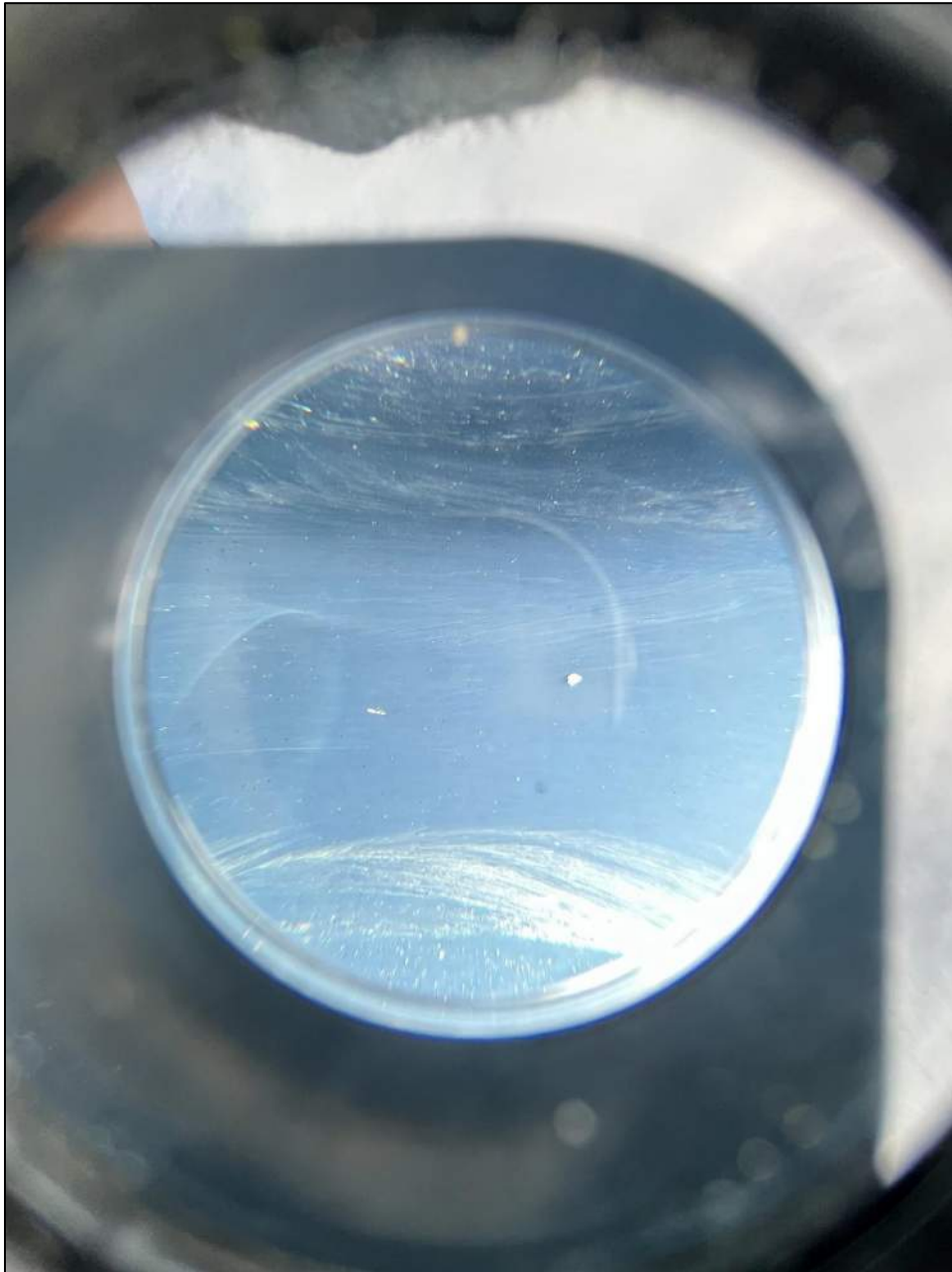
Photo 129: No coating disruptions were observed at the hail dents and spatters.
