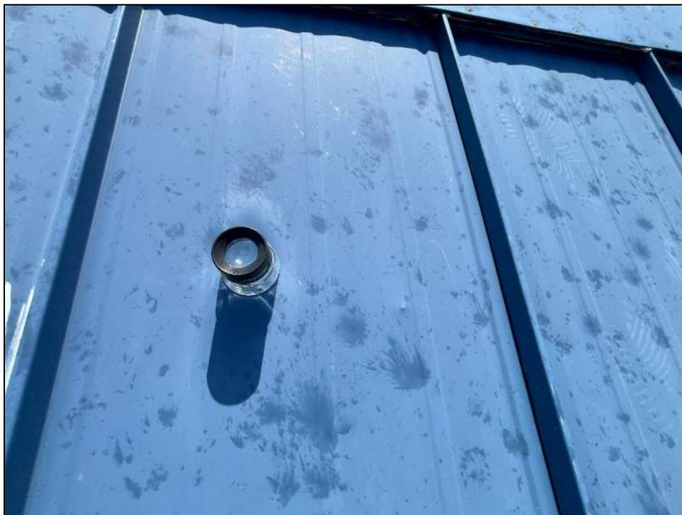
Photo 16: Microscope inspection indicated no coating disruption at hail dents or spatters.
