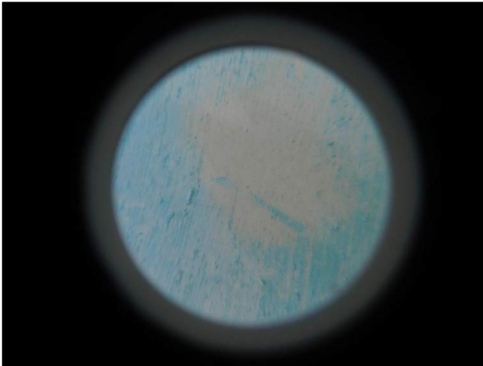
Photo 14: No coating disruption accompanied the hail denting in the closure metal surfaces.
