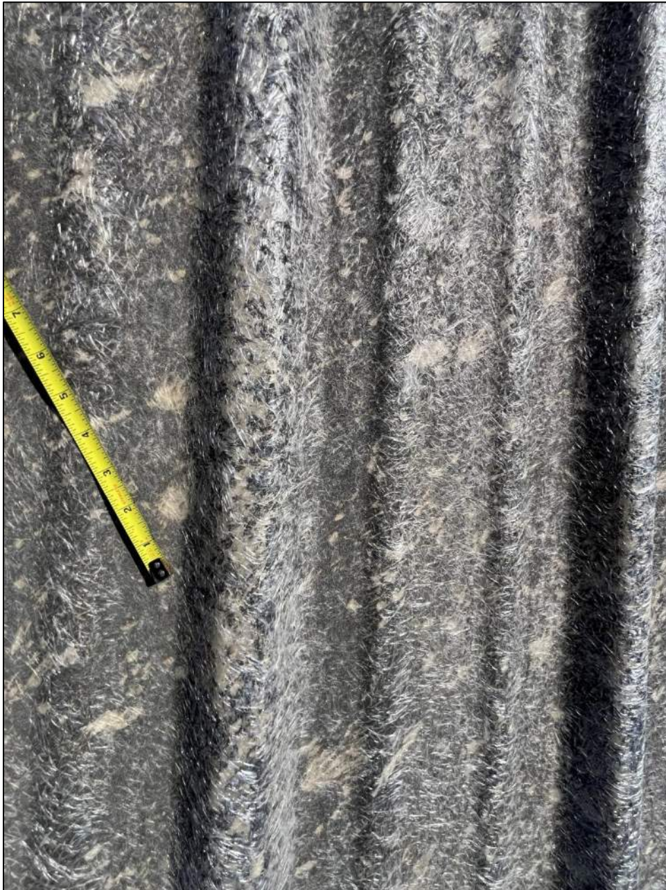
Photo 94: Skylight panels were not fractured at the spatters.
