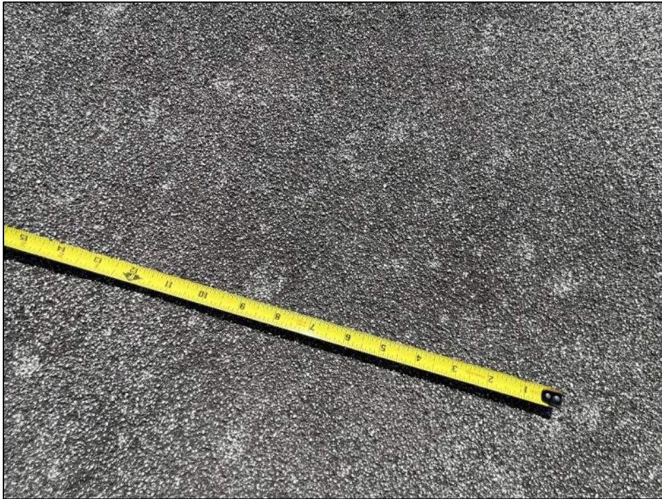
Photo 44: Largest hail spatter measured 1.13 inches (1-1/8) wide.
