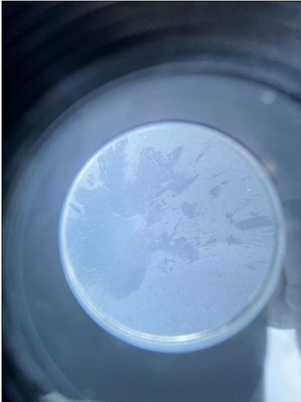
Photo 20: Microscope inspection indicated no coating disruption at hail dents or spatters.
