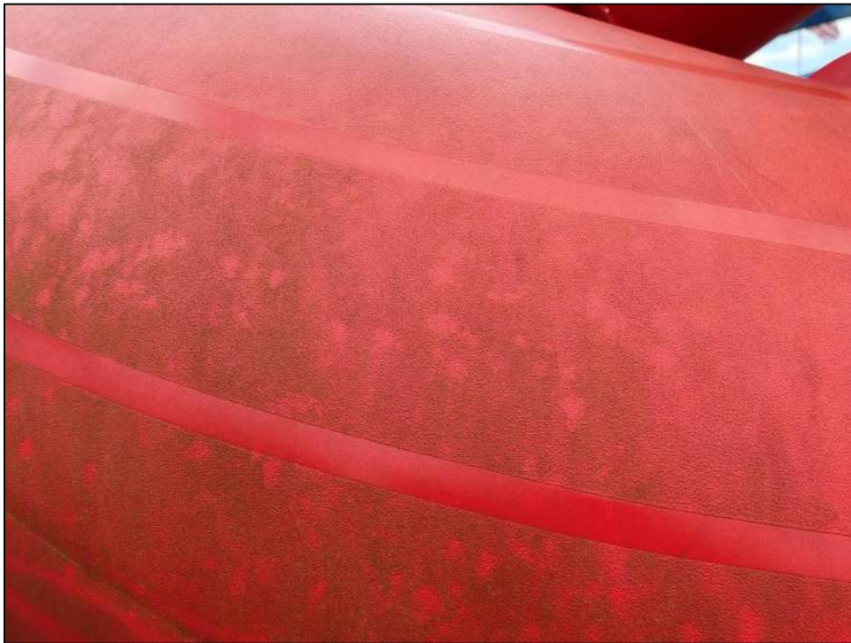
Photo 118: Top view of hail spatters on playset slides. No impact fractures were observed.
