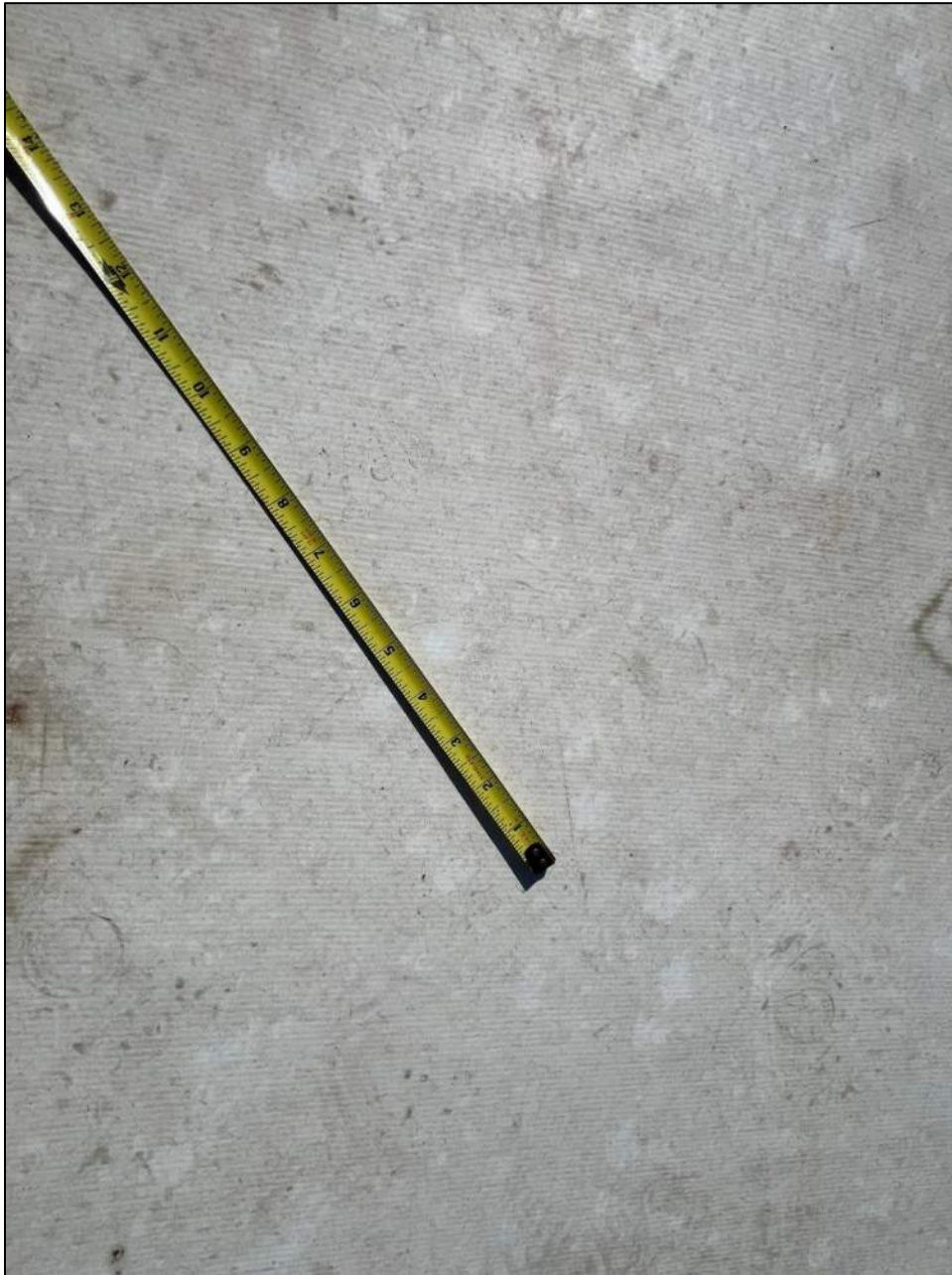
Photo 74: Largest hail spatters measured 1.0 inches in base width within the test square.
