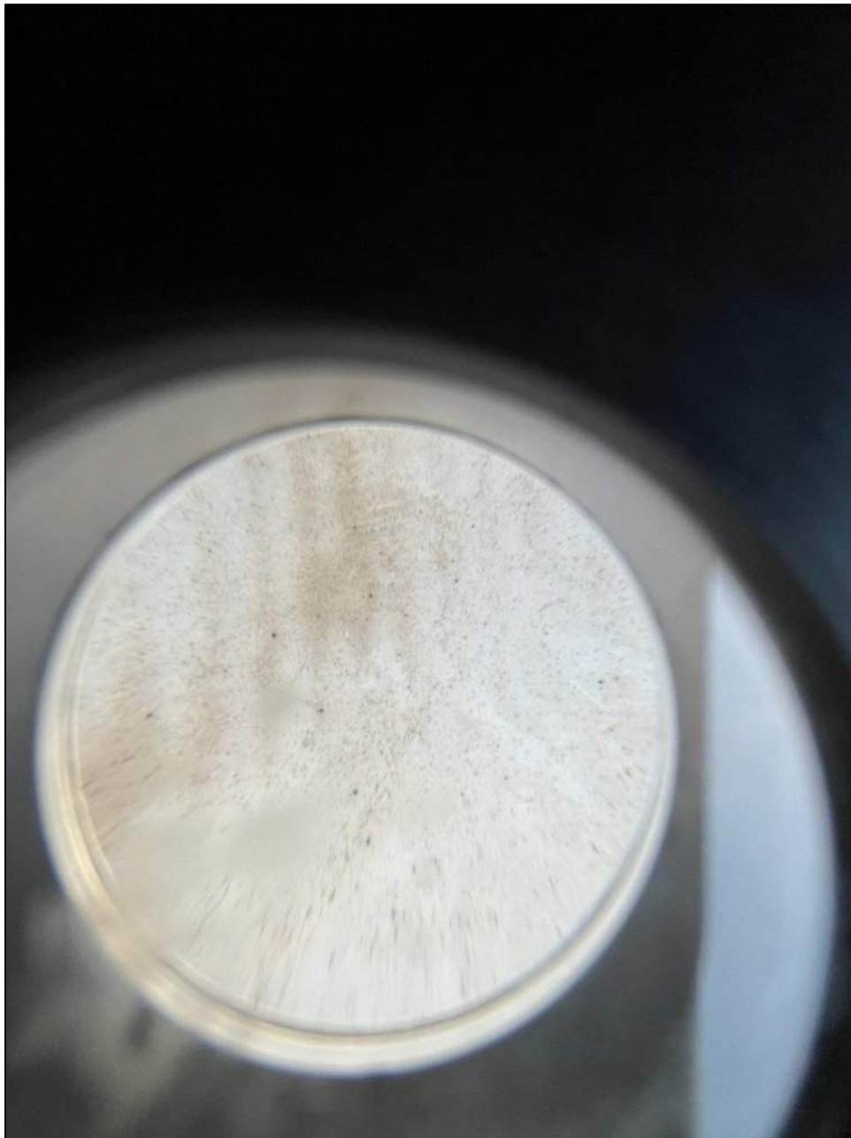
Photo 78: Microscope examination at the stress plates identified no PVC surface disruptions at spatters.
