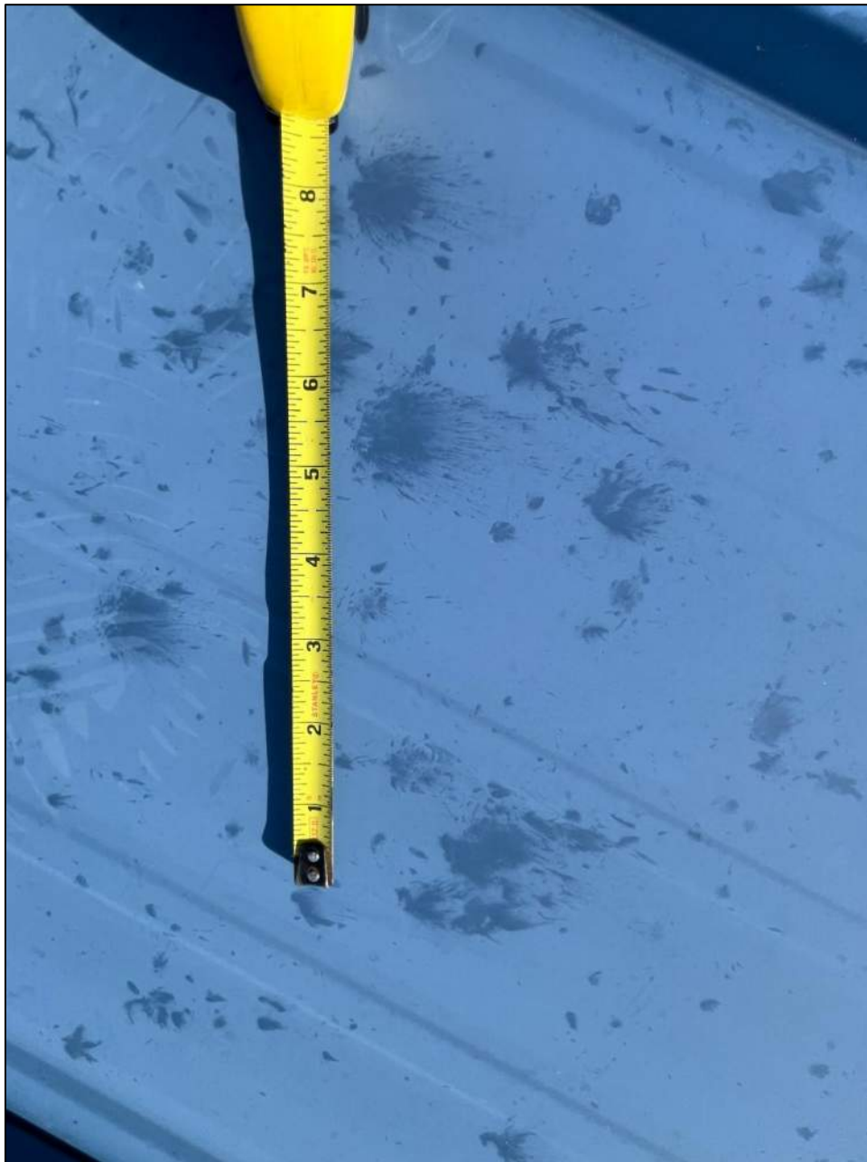
Photo 12: Largest hail spatter reflected up to 1.5-inch hail at this site.
