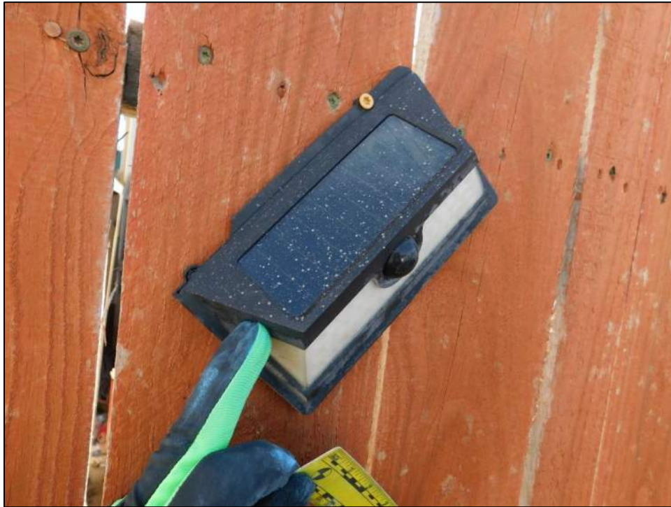
Photo 17: Solar light fixture on nearby fence walls was not fractured.
