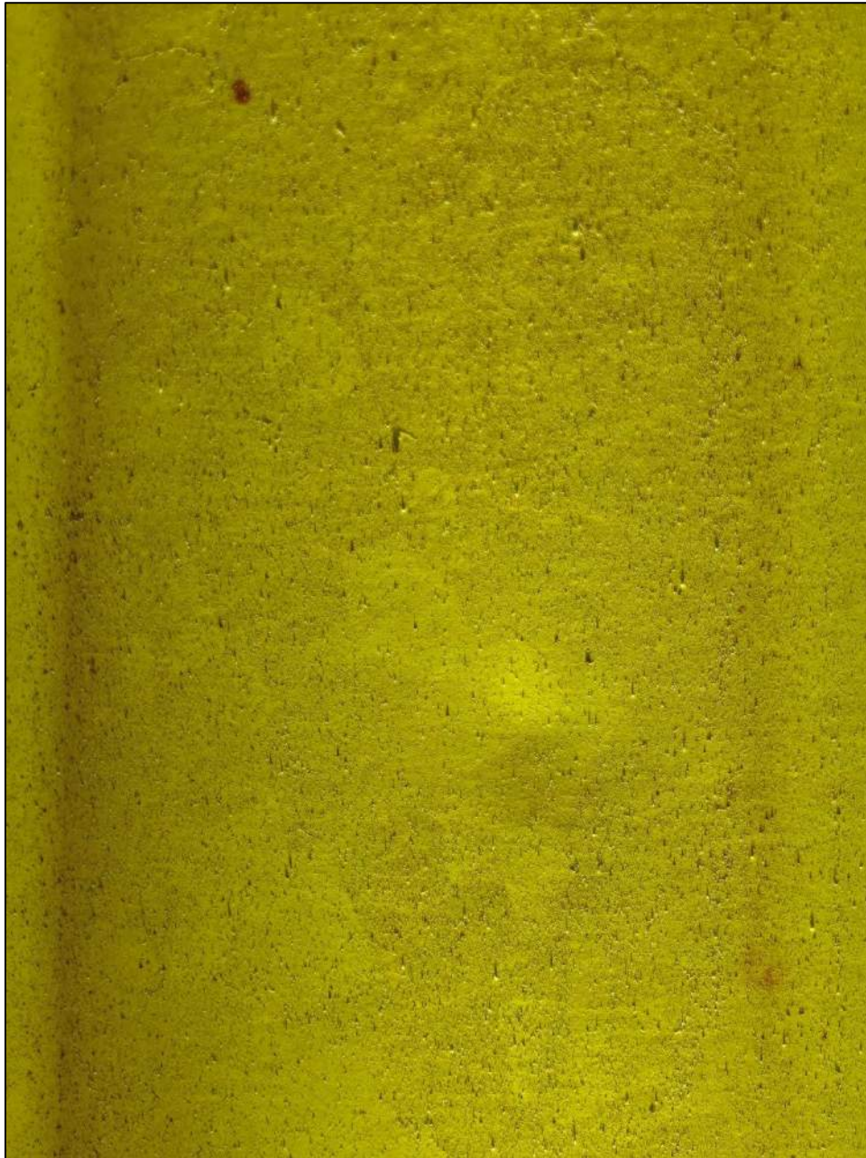
Photo 92: Dust pattern remained undisturbed at select dents.
