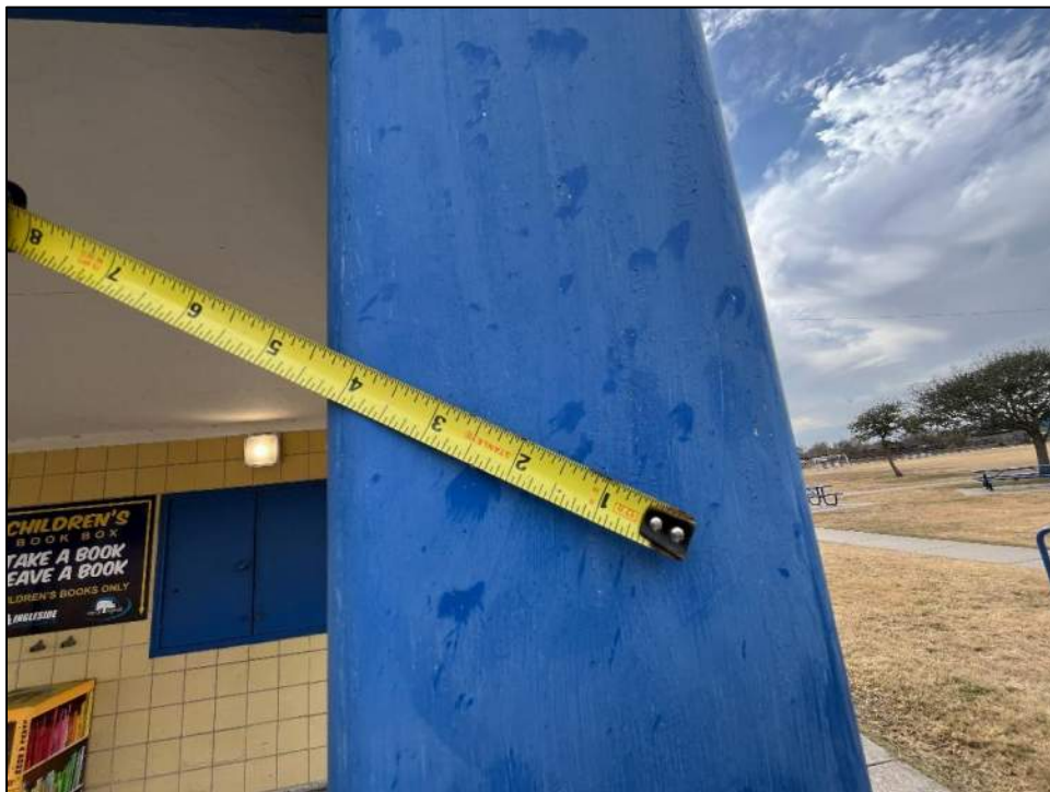
Photo 61: Hail spatters indicative of 0.75- to 1.0-inch hail.
