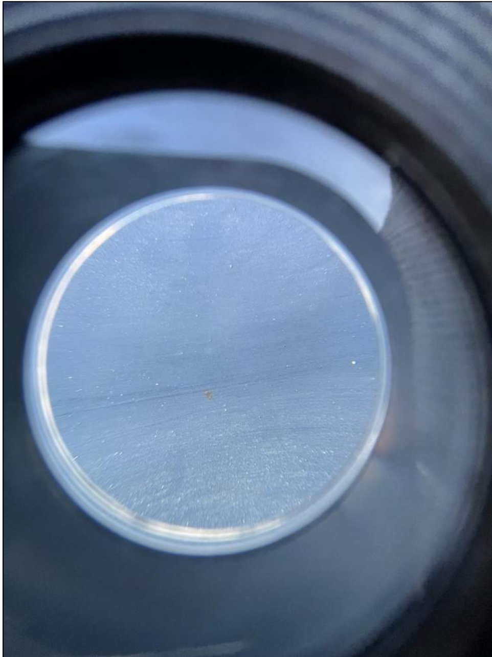
Photo 16: No coating disruptions were observed at the hail spatters.
