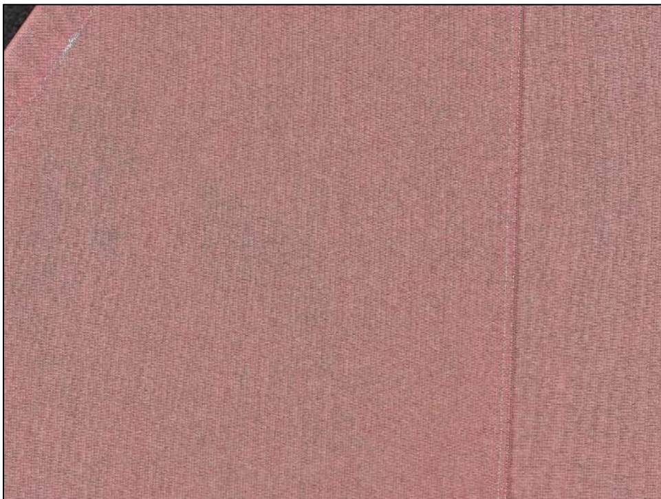
Photo 100: Close-up of the fabric. No fractures consistent with hail impact were observed.
