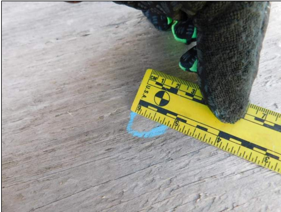
Photo 39: Hail spatters on nearby horizontal plywood surface resulted in no peck marks or wood grain disruptions.
