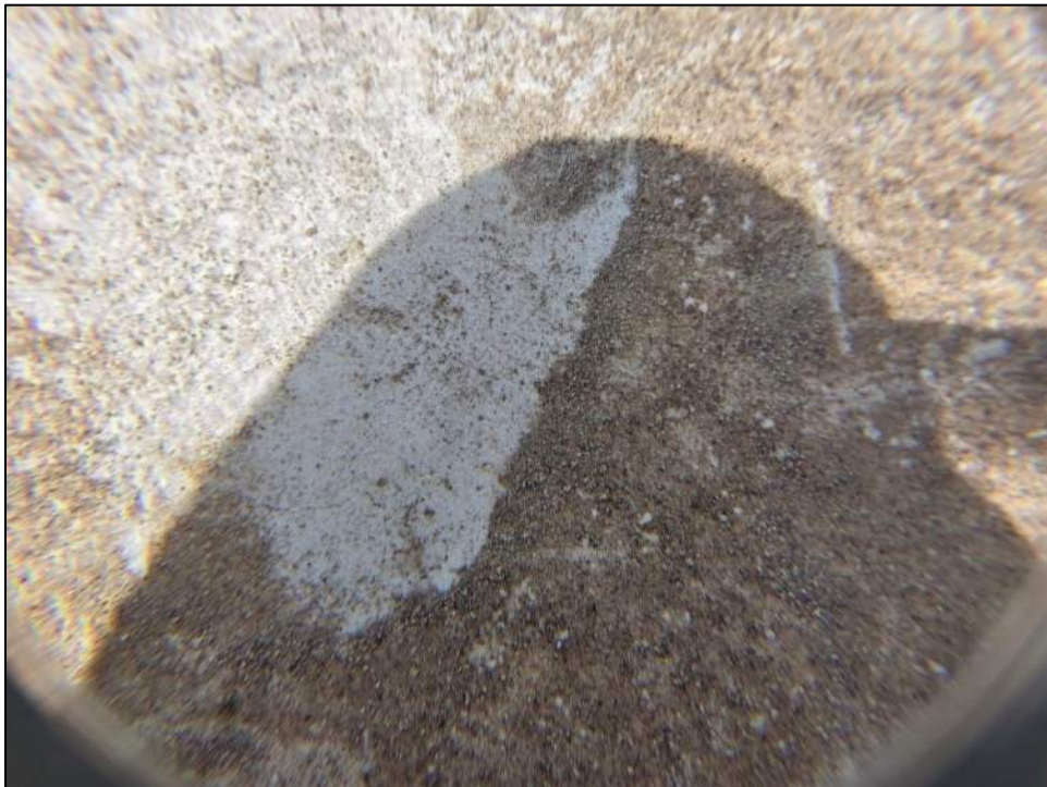
Photo 30: Microscope examination indicates no surface disruption at the spatter except for oxidation and grime displacement.
