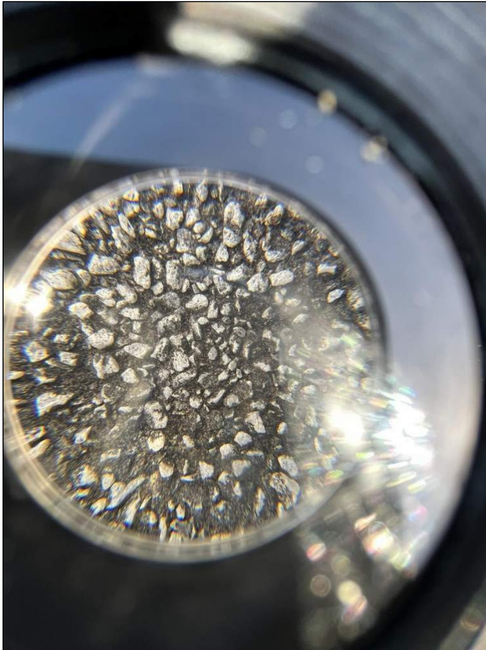
Photo 49: Microscope examination of the hail spatter exhibited no granule displacement due to hail impact.
